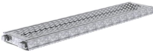
The working platform is created by laying two steel planks on top of the vertical frames. The steel planks are 32 cm wide and create a strong working platform. By placing the frames of the next lifts on top of the frames that bear the steel, the steel planks are secured against lifting up.
