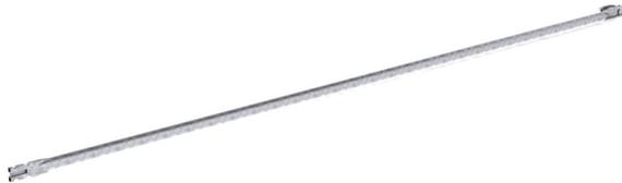
The vertical brace absorbs the horizontal loads that come into the scaffold construction. The vertical brace stabilizes the outer plane, parallel to the façade.
