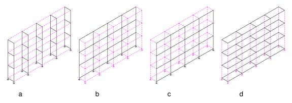
Figure 5.1: Sections of facade scaffold
